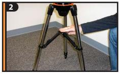
Assemble tripod by spreading the legs out until the center leg brace is fully extended.
